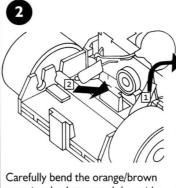
Carefully bend the orange/brown capacitor back to reveal the guide blade clip. Unclip the rear of the guide blade by pressing BACK & DOWN on the clip from the inside of the chassis with a SCREWDRIVER.
