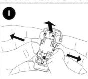
After a while, the pick-up braids underneath the cars may become worn out and need replacing. To do this, turn the car over and unclip the body from the chassis.
