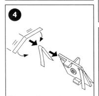
Fit new braids to replacement guide plate. The braids should be folded so that the ends on top of the guide plate are 10mm long.
