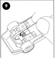
Periodically, oil the axle bearings and gear wheel with one drop of light machine oil.
