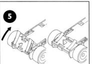
Fit the assembled guide plate assembly on to the chassis by engaging the front clip first and then the rear clip.
