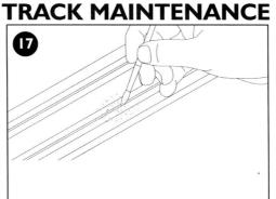
Keep the slot between the pick-up rails free from anything which would prevent the guide fin from travelling along it freely.
