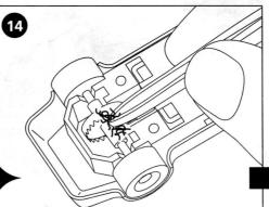
Remove any carpet fibres, pet hairs etc., from around the car's axles and gear wheel.
