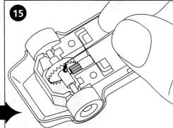
Periodically, oil the axle bearings and gear wheel with one drop of light machine oil.
