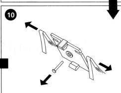
Remove the worn braids and guide pin from the braid plate.
