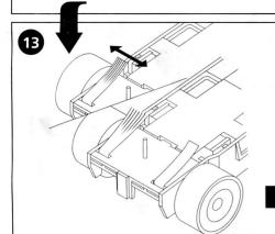
Refit the car body and tease out the ends of the braids so they make good contact with the pick-up rails in the track.
