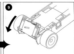
Turn the chassis over and remove the braid plate from its front clip.
