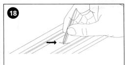
Make sure anything made of metal does not bridge the two pick-up rails which would cause a short-circuit.
