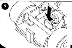
Unclip the rear of the braid plate by pressing down on the clip, from inside the car, as shown in the diagram. You may have to use a screwdriver to do this.
