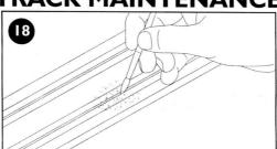
Keep the slot between the pick-up rails free from anything which would prevent the guide pin from travelling along it freely.
