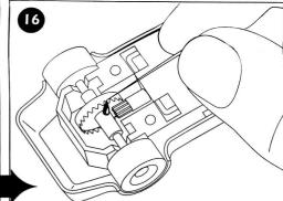
Periodically, oil the axle bearings and gear wheel with one drop of light machine oil.
