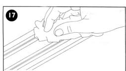
Always keep track clean by wiping over with a non-fluffy cloth, especially before putting the set away. Keep the pick-up rails shiny by rubbing carefully with a nylon "Scotch" washing-up pad or track cleaning rubber, reference R8087, obtainable from Hornby stockists.
