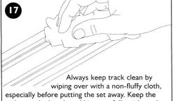
pick-up rails shiny by rubbing carefully with a nylon "Scotch" washing-up pad or track cleaning rubber, reference R8087, obtainable from Hornby stockists.
