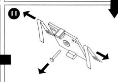
Remove the worn braids and guide pin from the
