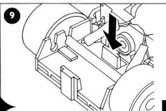
Unclip the rear of the braid plate by pressing down on the clip, from inside the car, as shown in the diagram. You may have to use a screwdriver
