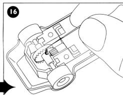
Periodically, oil the axle bearings and gear wheel with one drop of light machine oil.
