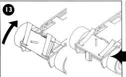
Fit the assembled guide plate assembly on to the chassis by engaging the front clip first and then the
