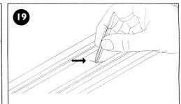
Make sure anything made of metal does not bridge the two pick-up rails which would cause a short-circuit.
