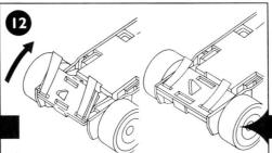
Fit the assembled guide plate assembly on to the chassis by engaging the front clip first and then the rear clip.
