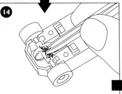
Remove any carpet fibres, pet hairs etc., from around the axles and gear wheel.
