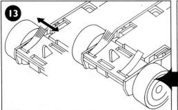
Refit the skateboard and tease out the ends of the braids so they make good contact with the pick-up rails in the track.
