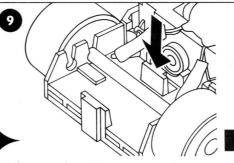
Unclip the rear of the guide plate by pressing down on the clip, from inside the chassis, as shown in the diagram. You may have to use a screwdriver to do this.
