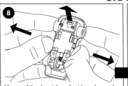
After a while, the pick-up braids underneath the skateboards may become worn out and need replacing. To do this, turn the skateboard over and unclip from the chassis.
