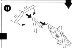
Fit new braids to the replacement guide plate. The braids should be folded so that the ends on top of the guide plate are 10mm long.
