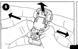
After a while, the pick-up braids underneath the cars may become worn out and need replacing. To do this, turn the car over and unclip the body from the chassis.
