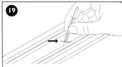
Make sure anything made of metal does not bridge the two pick-up rails which would cause a short-circuit.
