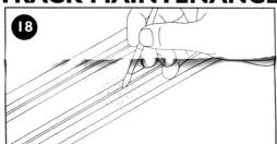
Keep the slot between the pick-up rails free from anything which would prevent the guide pin from travelling along it freely.
