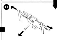
Remove the worn braids and guide pin from the braid plate.
