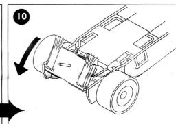
Turn the chassis over and remove the braid plate from its front clip.
