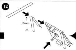
Fit new guide pin and braids to the braid plate. The braids should be folded so that the ends on top of the guide plate are 10mm long.
