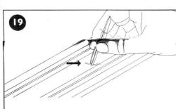
Make sure anything made of metal does not bridge the two pick-up rails which would cause a short-circuit.
