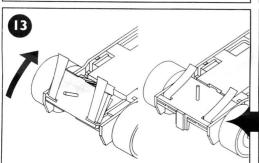
Fit the assembled guide plate assembly on to the chassis by engaging the front clip first and then the rear clip.
