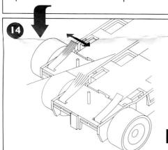
Refit the car body and tease out the ends of the braids so they make good contact with the pick-up rails in the track.
