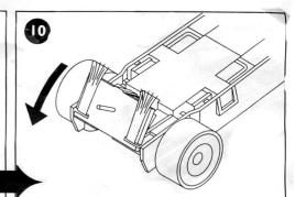
Turn the chassis over and remove the braid plate from its front clip.
