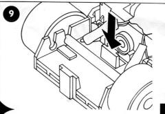
Unclip the rear of the braid plate by pressing down on the clip, from inside the car, as shown in the diagram. You may have to use a screwdriver to do this.
